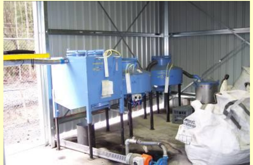
Ankur Gasifier dual firing a diesel genset - Huon Valley, Tasmania.
