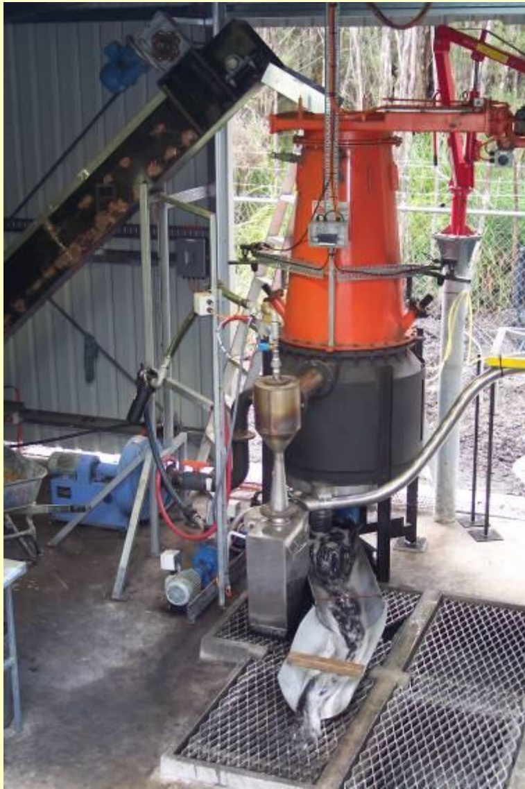
Ankur Gasifier dual firing a diesel genset - Huon Valley, Tasmania.
