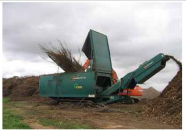
Figure 4 – Horizontal rotary hogger, self-propelled, requires loader to infeed raw material
