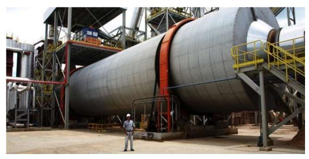
Workplaces that manufacture engineered wood products or wood pellets may be at risk of fire, deflagration or explosion due to the buildup of combustible off-gas within dryers and associated drying systems during the process of drying wood fibre.
