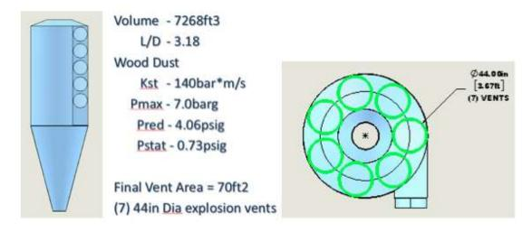
As we can see while all (7) explosion vents will fit on the top of the cyclone, you end up have explosion vents installed in the high flow area within the cyclone.
