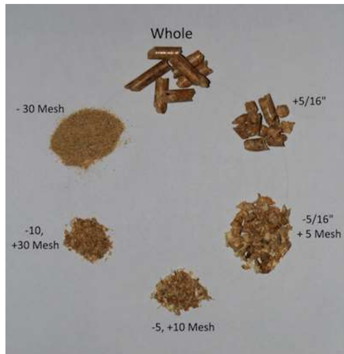
Figure 2: wood pellet particle size distribution samples during processing (from Paul Janzé – Advanced Biomass Consulting Inc. November 2, 2014).
