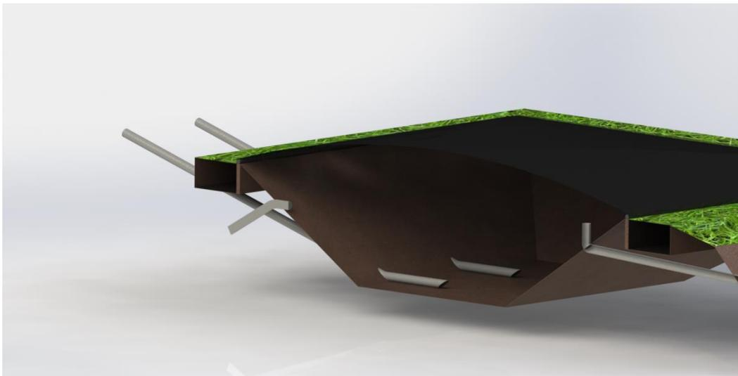
Figure 28: Cross section view of Digester
