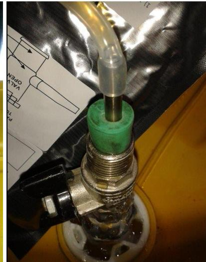
Figure 20: Photo of Leak around gas outlet
