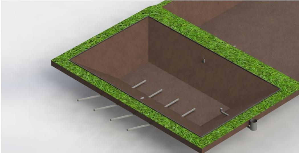
Figure 27: Close up view of Digester uncovered, showing sludge removal pipes, level drum and linking pipe
