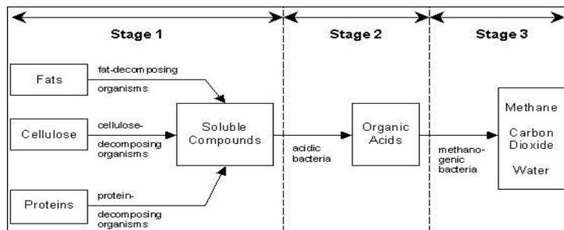
Figure 3: Biological Process for Anaerobic Digestion
