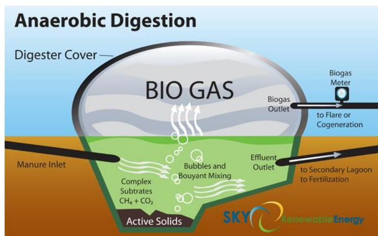
Figure 2: Anaerobic Digestion (Sky Renewable Energy, 2012)
