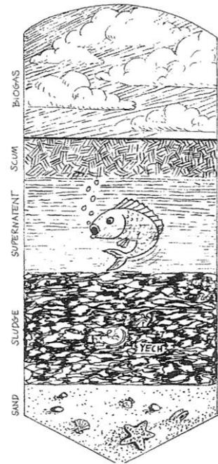
Figure 1: Anaerobic Pond Layers
