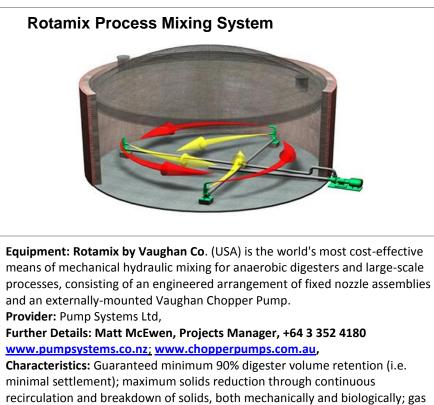
recirculation and breakdown of solids, both mechanically and biologically; gas production maintained to levels seen at system start with no drop-off; integrated scum and foam protection available; no moving or rotation parts within the process ensure a minimum of maintenance; 10 year mixing nozzle warranty against wear and corrosion.
