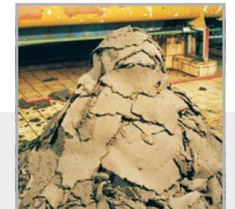
Sewage sludge dewatered by a chamber filter press: Solids content > 35 % DS
