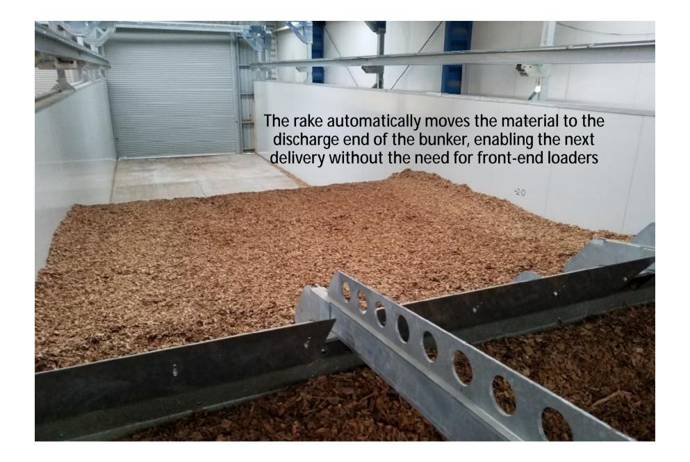
It is always seeking to maximize the storage area in the bunker. The Toploader screen shows the latest volume. Supplier sees when more can be delivered.
