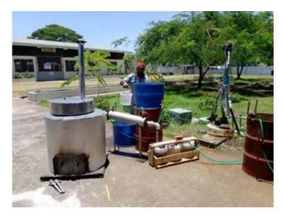
The system consists of a retort (left) fired typically by wood or fuel from the process. The retort will take around 7kgs of mixed Polyethylene and PET. The pyrolysis gases pass through a condenser (center left with cooling water in drum behind) with crude accumulating in the containers (center right). The incondensable gas (mainly methane/ethane mix) is stored in a water sealed system (right).
