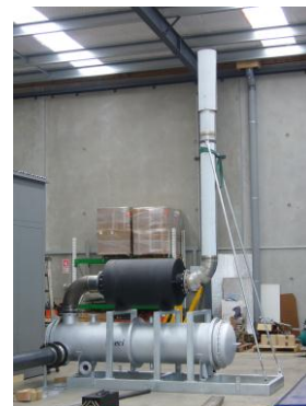
Exhaust heat recovery unit
