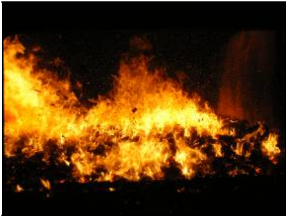
Wood chip blend, grate low fire.
