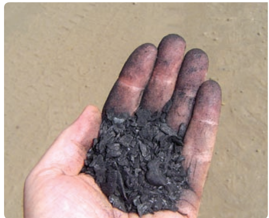
Char generated through the gasification process.
