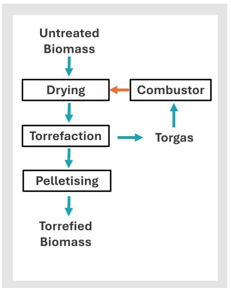
Torrefaction is a thermal treatment process which transforms biomass, in this case wood, into a coal-like material by heating it without oxygen at temperatures generally ranging from 200–300°C.
