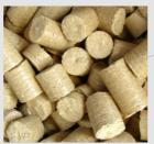
Torrefaction of wood significantly increases the energy density of the product.
