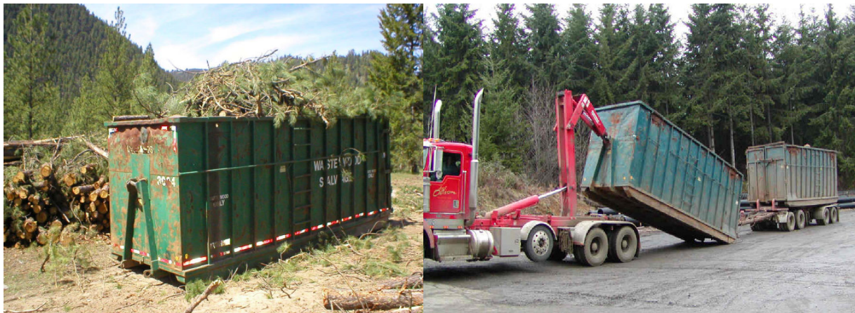
Figure 3 - set-out bins (left) and hook truck and trailer (right)
