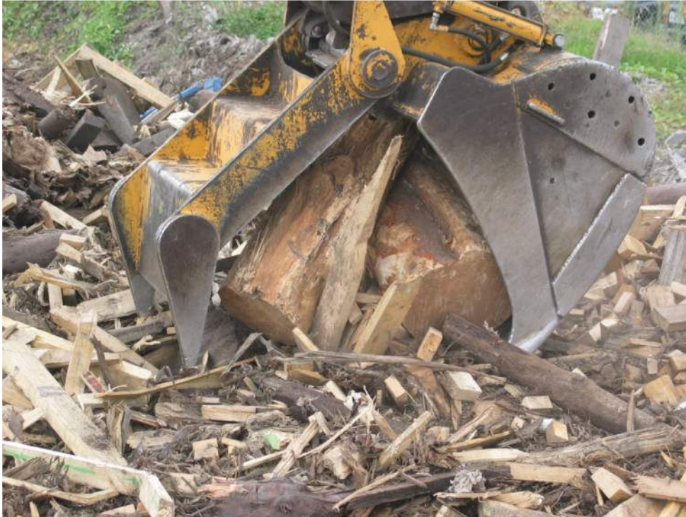
Figure 12 – excavator bucket fitted with hydraulic thumb
