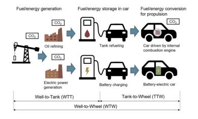
Figure 9: Well to tank vs Well to Wheel emissions<sup>27</sup>
