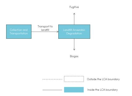
Figure 5: LFG to gaseous biofuel LCA Upstream Boundary
