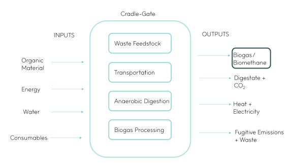
Figure 8: Biogas / Biomethane Process Flows example inputs and outputs.
