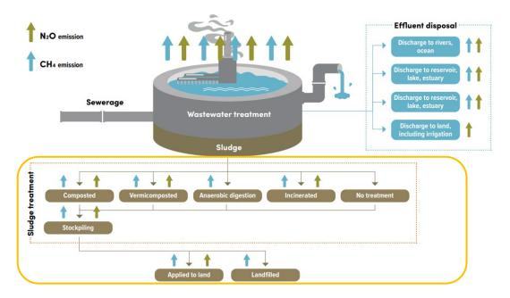
Figure 6: Biogenic methane and nitrous oxide emissions from wastewater treatment, picture credit Navigating to Net Zero, Water NZ, Wastewater emissions<sup>20</sup>.
