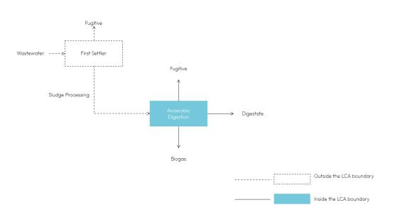
Figure 7: WWTP AD Plant for Treatment of Sludge showing upstream project boundary.
