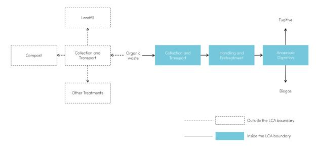
Figure 4: Organic Waste Diversion to AD Plant, Upstream LCA System Boundary<sup>14</sup>
