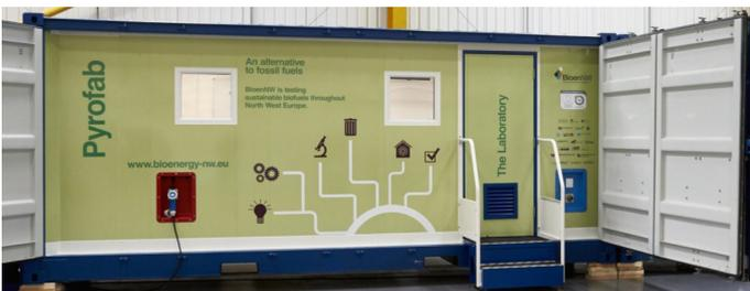
**Figure 1:** Mobile containerised Pyrofab based on Pyroformer™ technology developed by EBRI at Aston University.
