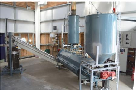
**Figure 1:** Pilot-scale pyrolysis unit (50kg/h).
