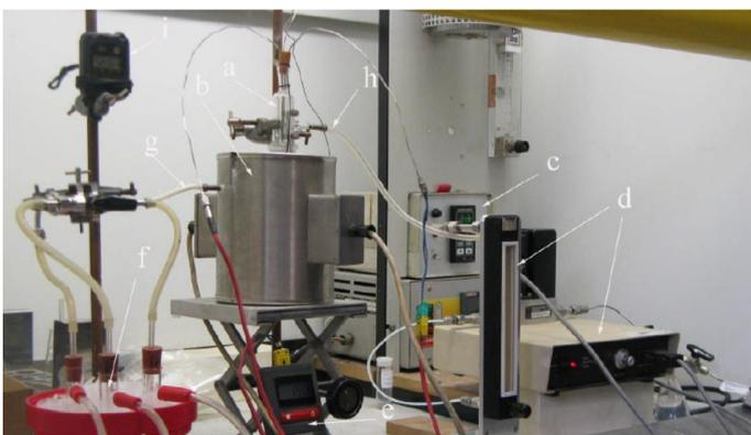
Figure 1: Bench scale experimental rig for catalytic pyrolysis.
