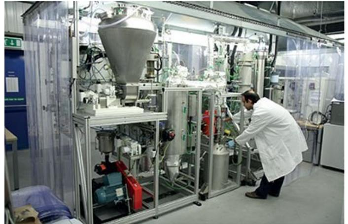
**Figure 2:** 5 kg/h fluid bed pyrolysis rig for Future Blends, UK.
