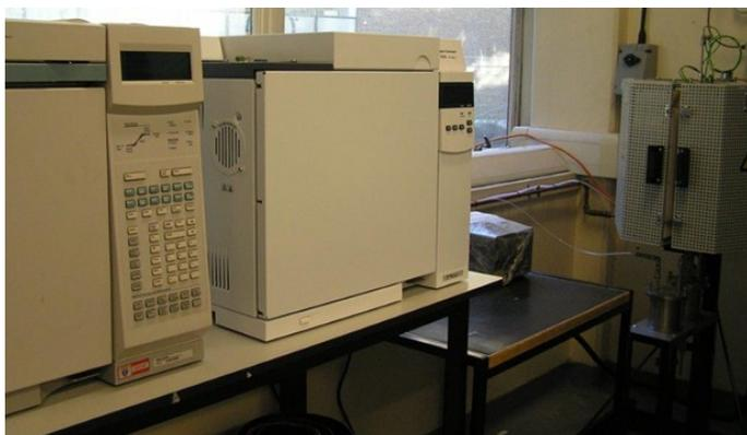
Figure 1: Pyrolysis equipped with online GCs.
