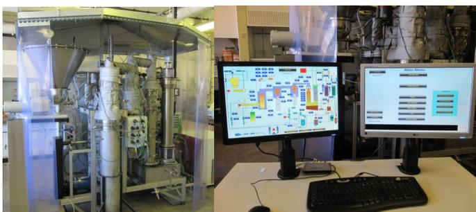
**Figure 1:** (Left) Completed 5 kg/h (dry biomass input) rig overhaul, UK; (Right) New PLC system for pyrolysis rig.
