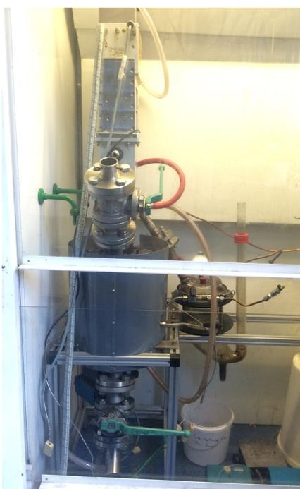
Figure 1: Laboratory scale microwave heated pyrolysis apparatus.
