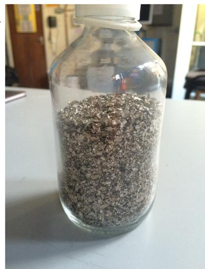
Figure 2: Aluminium recovered from laminated beverage packaging.
