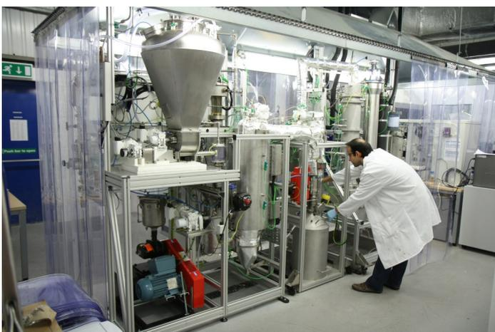
Figure 1: 5 kg/h fluid bed pyrolysis rig.
