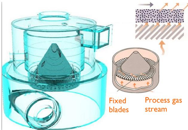
**Figure 1:** The TORBED<sup>®</sup> Compact Bed Reactor (CBR). Gas is introduced underneath the blades of the CBR leading to high velocity gas jets that fluidise and fully mix the bed maximising gas-solid contact.
