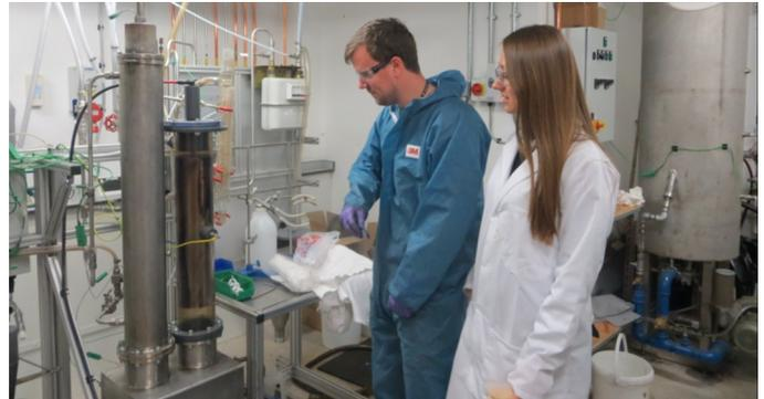
**Figure 2:** Aston's 1kg h<sup>-1</sup> continuous fast pyrolysis unit.
