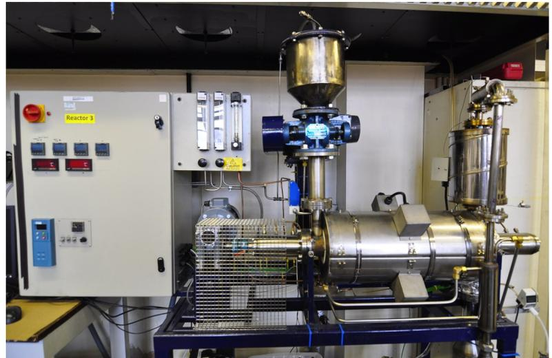
**Figure 1:** Screw kiln pyrolysis-gasification reactor.
