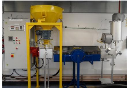
**Figure 2:** Continuous screw pyrolysis unit (5kg/h).
