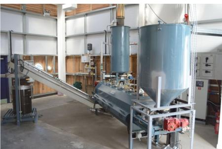
**Figure 1:** Pilot-scale pyrolysis unit (50kg/h).
