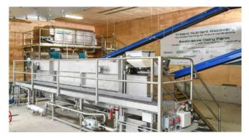
and used for cow bedding. Additional processing and de-watering on-site then create a nutrient-rich cake (approx. 25% solids) that is used as fertilizer for cropland located 30-minutes away. The separated liquid portion (similar to a low nutrient tealike water) is either irrigated onto the farm's nearby crops and/or used as flush-water in their manure handling system. The nutrient recovery system is the start of the feedback loop of the P and N cycles of a circular economy.
