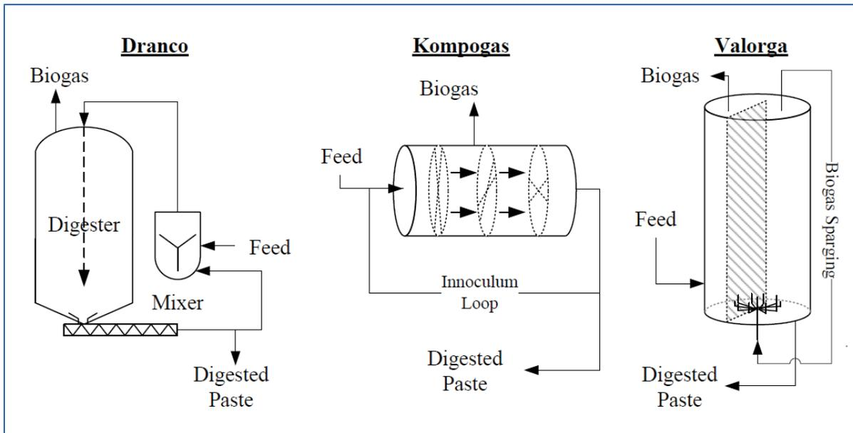
**Figure 11:** Solid-waste (dry) digester design: (a) Dranco, (b) Komlogas and (c) Valorga
