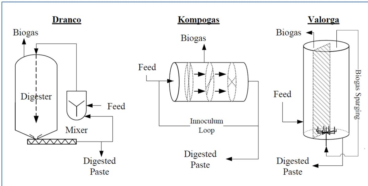
**Figure 11:** Solid-waste (dry) digester design: (a) Dranco, (b) Kompogas and (c) Valorga
