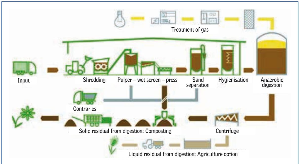
**Figure 10:** Process chain of a wet AD plant treating biowaste
