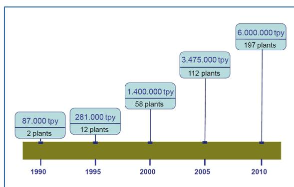
**Figure 9:** Development of AD plants for MSW digestion in Europe<sup>11</sup>
