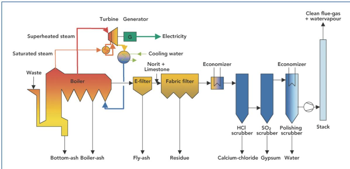
Figure 17: Layout of the high-efficiency WFPP scheme, Amsterdam
