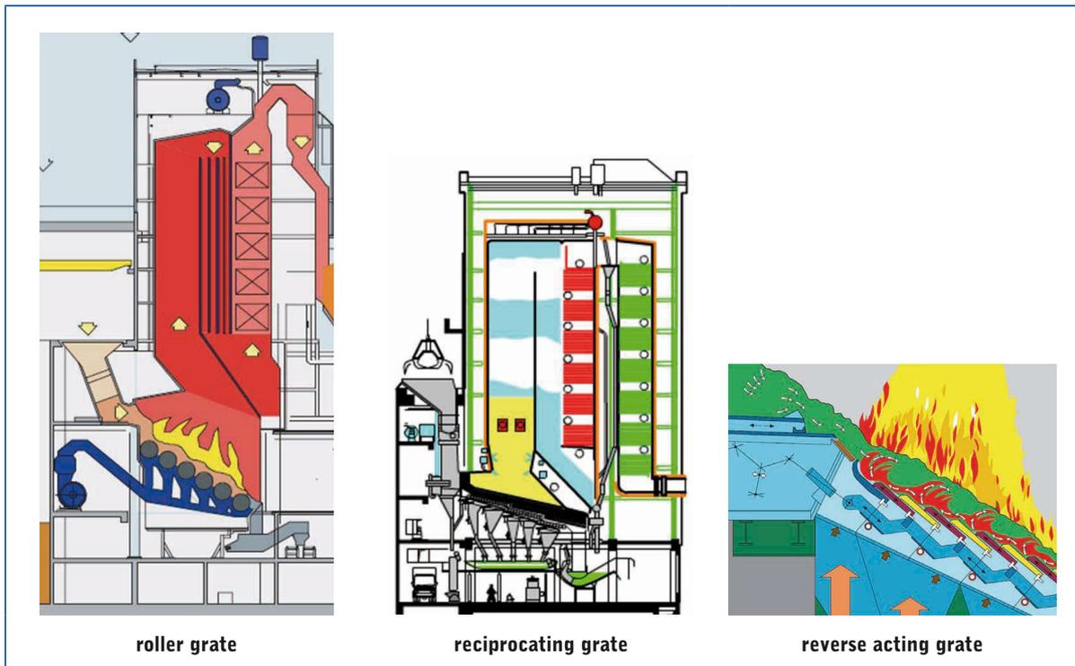
**Figure 15:** The three basic designs of grate furnaces: roller (left), reciprocating (central), reverse-acting grate (right)
