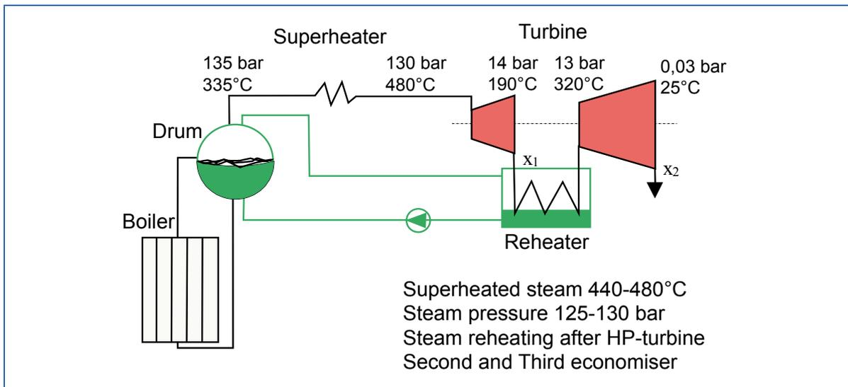
Figure 18: Intermediate steam reheating system
