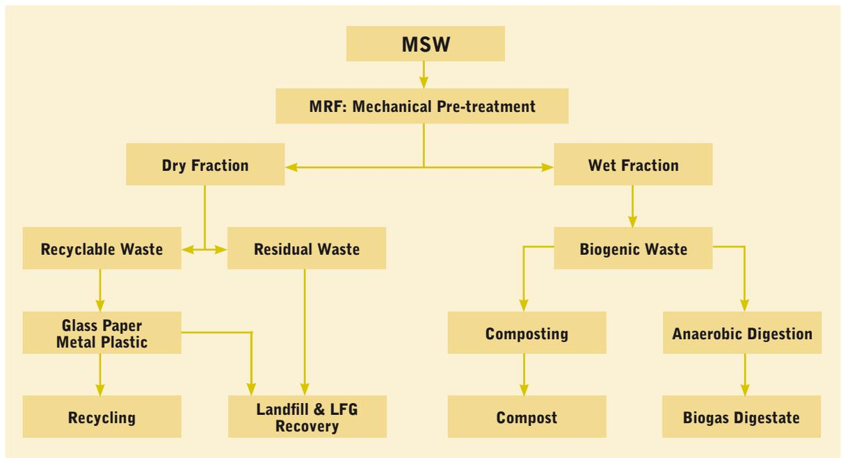
**Figure 1:** A typical dry-wet waste diversion model
