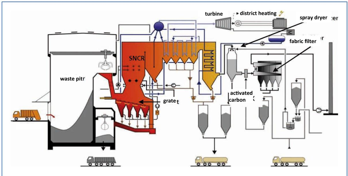
**Figure 16:** Stack gas treatment with SNCR, addition of activated carbon and fabric filter to remove NO<sub>x</sub>, dioxins and fly ashes
