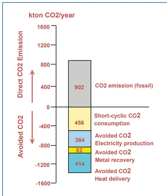
Figure 19: CO<sub>2</sub> emission of energy production vs CO<sub>2</sub> emission avoided through WtE and recycling
