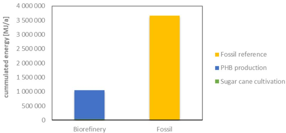
Figure 21 Cumulated energy demand of biorefinery compared to reference plant - case study 2.
