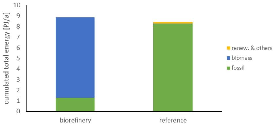
Figure 37 Cumulated energy demand of biorefinery compared to reference plant - case study 4.
