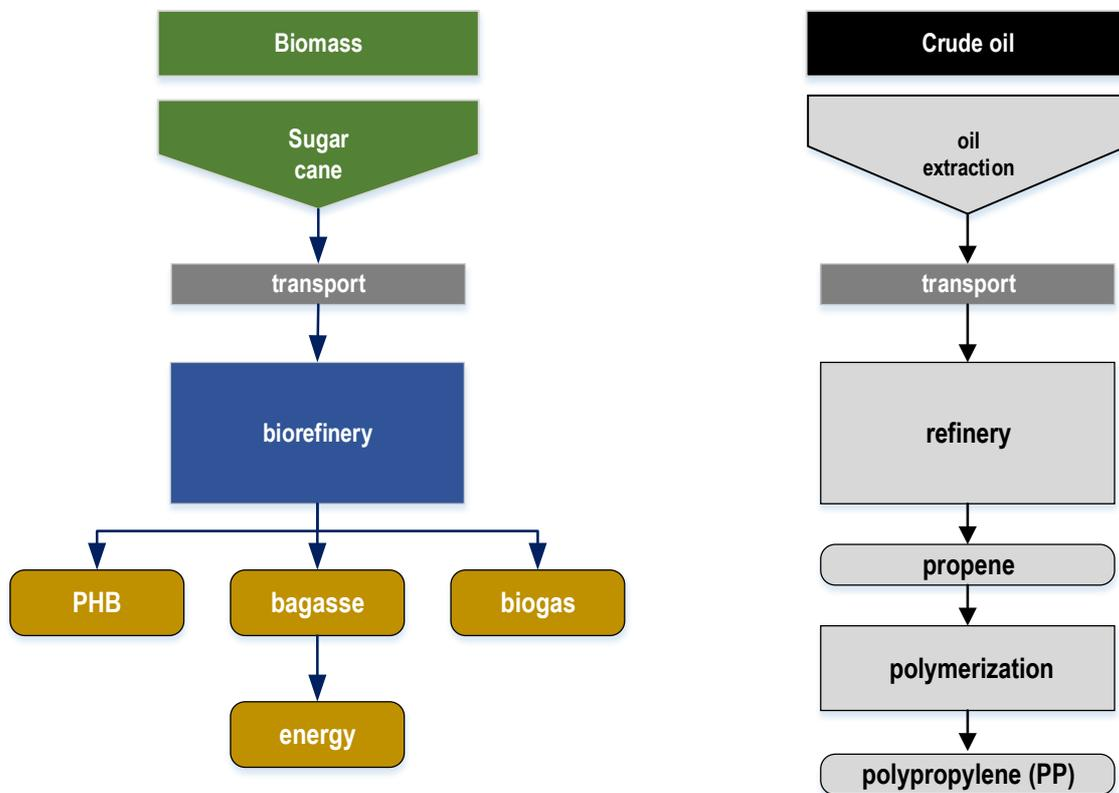
Figure 20 Biorefinery and reference system – value chain case study 2 (cradle to gate)
