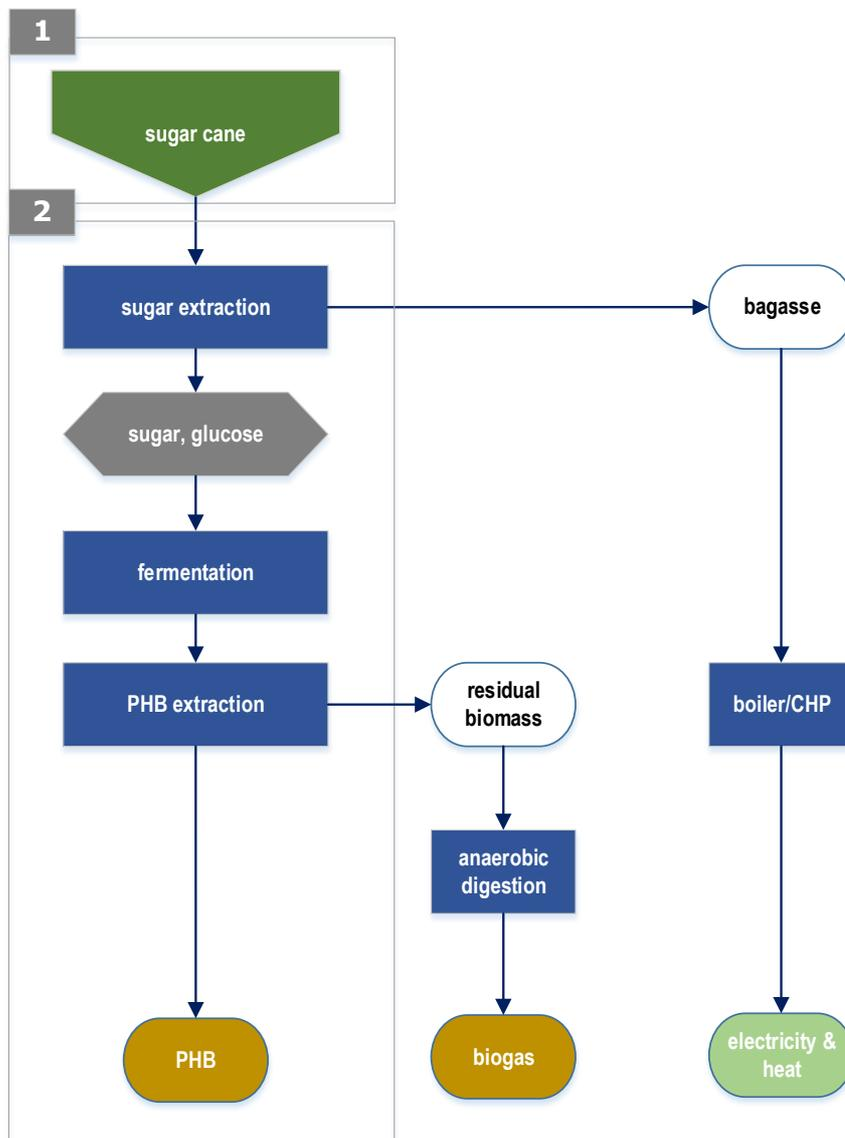
Figure 17 Poly-hydroxybutyrate (PHB) biorefinery pathway.
