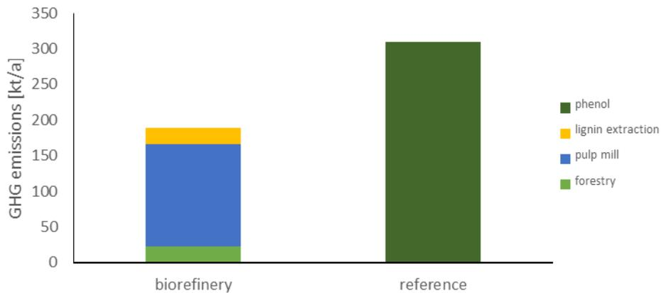
Figure 38 Greenhouse gas emissions of biorefinery compared to reference plant - case study 4.
