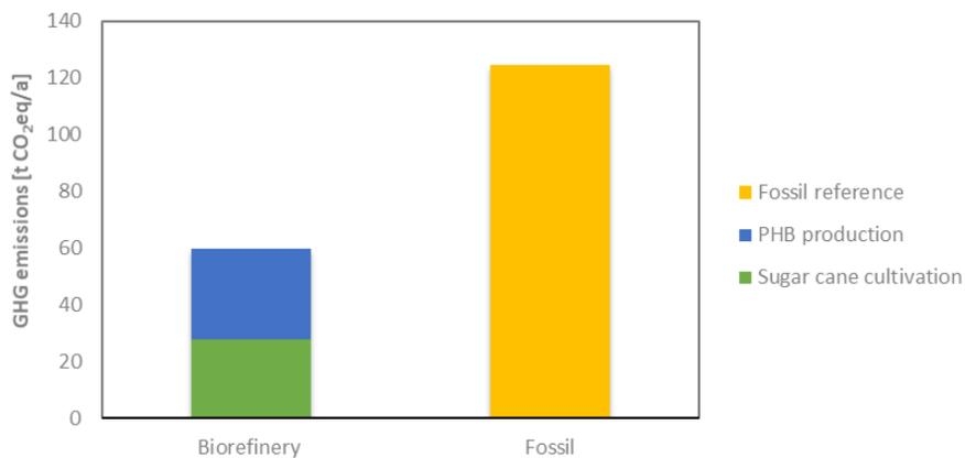
Figure 22 Greenhouse gas emissions of biorefinery compared to reference plant - case study 2.
