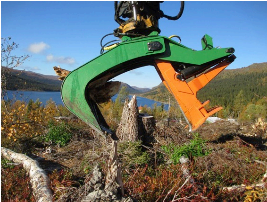
Figure 4.2. The TL-GROT AB stump head cuts the roots close to the stump and then lifts both the stump core and the coarse roots. Unfortunately, R&D momentum was lost before the head was fully developed, so it has not yet come into production.
