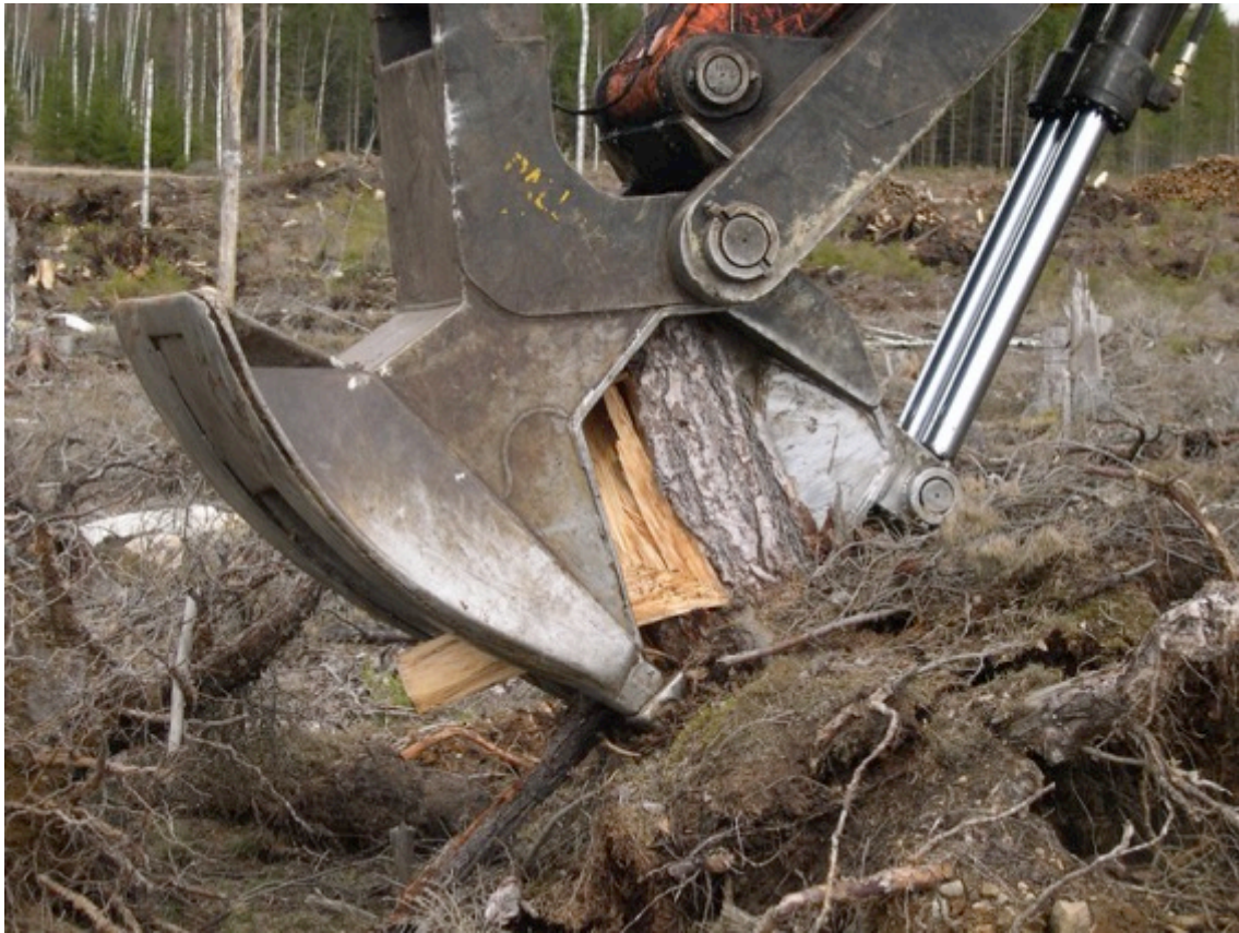
Figure 4.1. The Pallari 160 is a commonly used head for stump extraction in both Sweden and Finland. Two teeth grasp the stump from one side while a sharpened knife exerts pressure and cracks the stump from the other.
