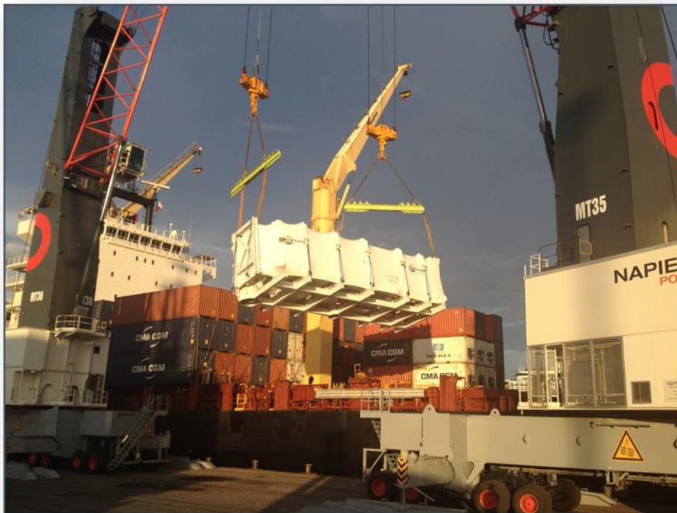
Boiler loading at Napier Port
