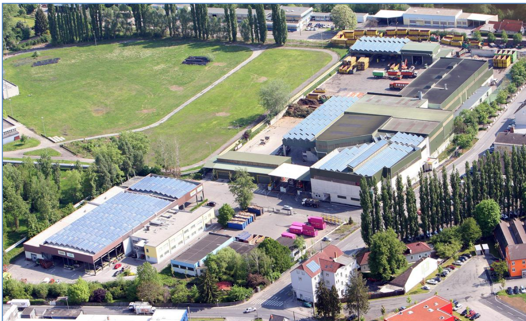
Figure 9: The solar thermal pre-heating system for the nearby AEVG gas thermal plant (beyond the left border of the photo) in Graz, Austria. Source: S.O.L.I.D. Gesellschaft für Solarinstallation und Design mbH
