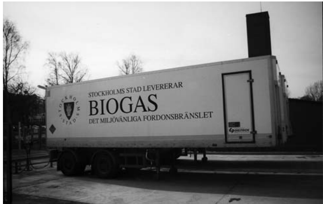
Picture 5: Trailer for transport of biogas to filling stations in Stockholm
