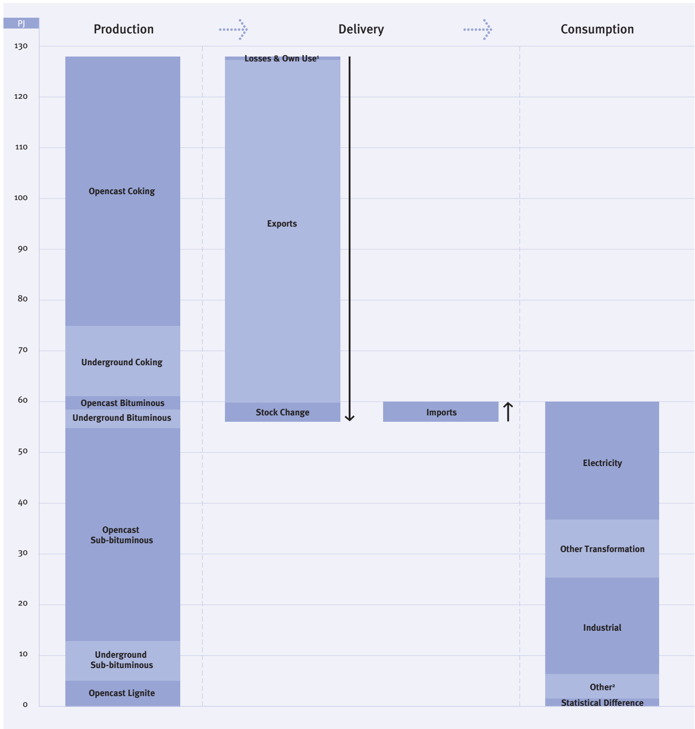
Figure C.6: Coal Energy Flow Diagram for 2011
