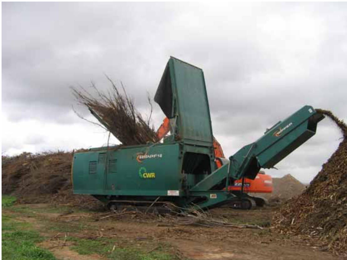
Figure 3 - CWR's Ripper working in 9 year old radiata pine, converting whole trees into boiler fuel (See Appendix I).
