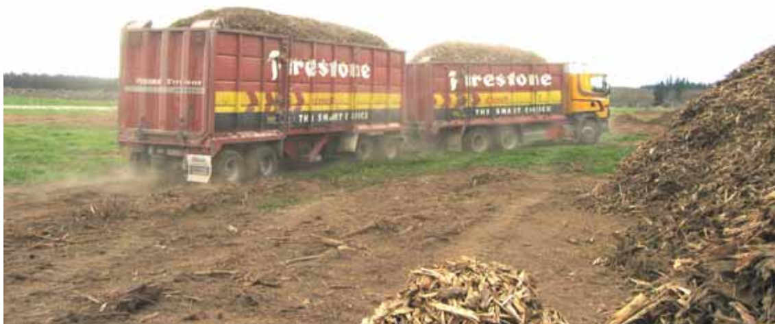
Figure 6 - Truck and trailer rig used for transporting processed residues from the processor to the energy plant
