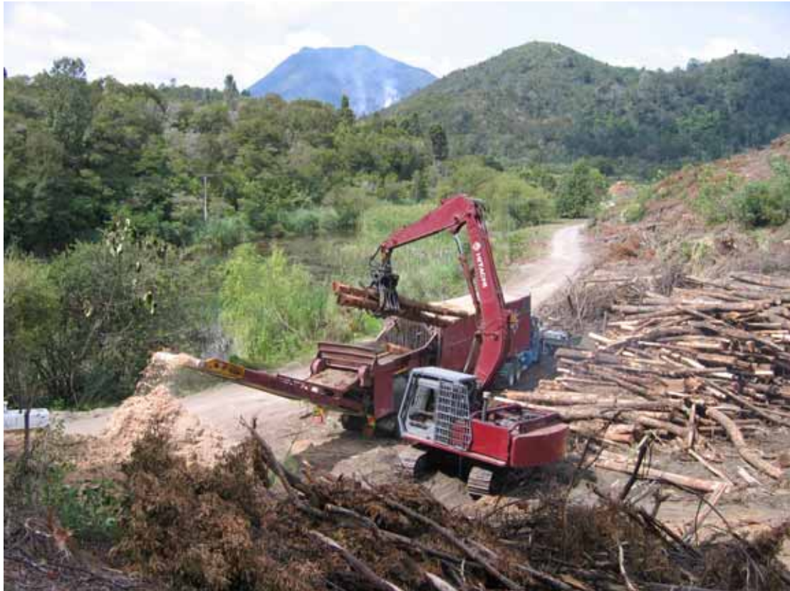
Figure 4 - Plateau Bark's WoodWeta converting reject logs and logging residues into boiler fuel (see Appendix II)
