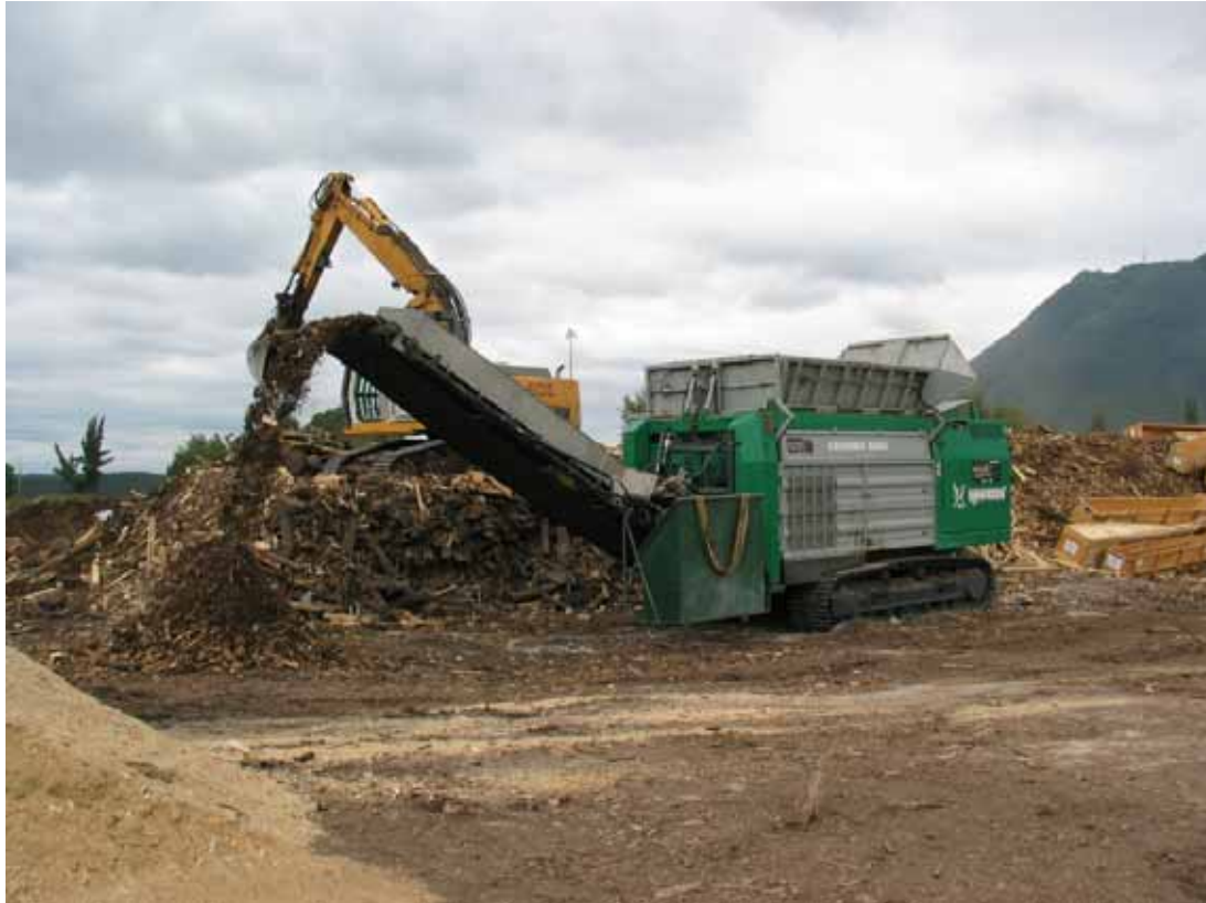
Figure III-1 – The Crambo 6000 processing wood waste into boiler fuel
