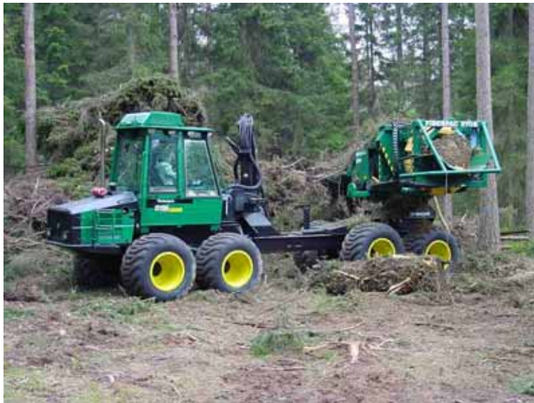
Figure 13 - Above, forest residue baler, forwarder mounted. Note the bale on the ground in front of the rear wheels.
