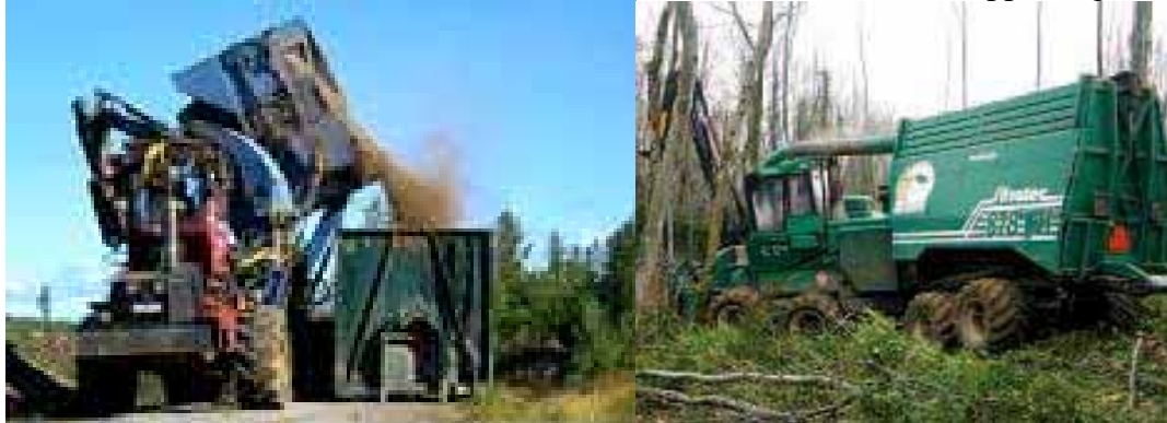
Figure 14 - Below, chipper forwarder and set-out bin (left), terrain chipper (right)
