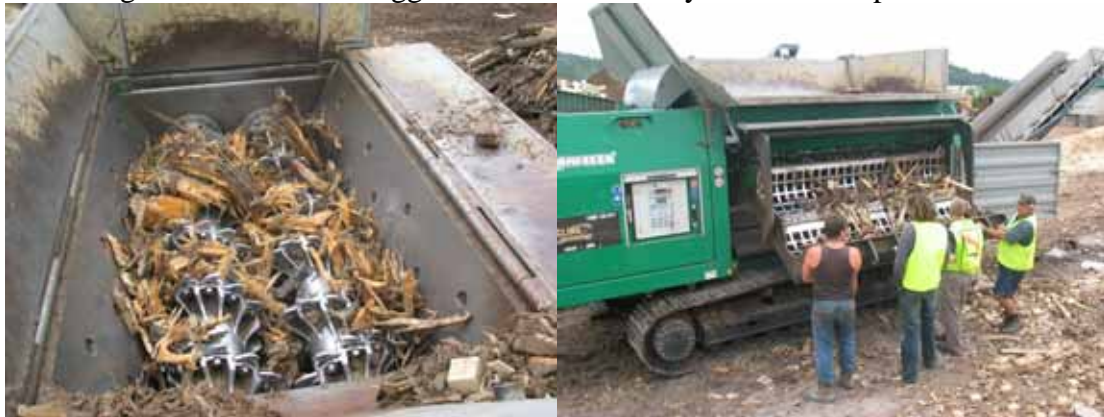
Figure III-4 - Hogging augers and knives (left) and sizing screens (right)
