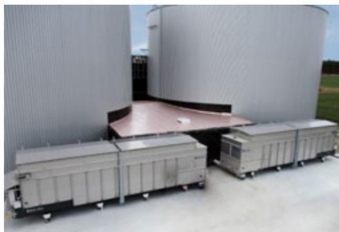
2 solid dosing systems type BIG-Mix 118 m<sup>3</sup> with a total capacity of 236 m<sup>3</sup>
