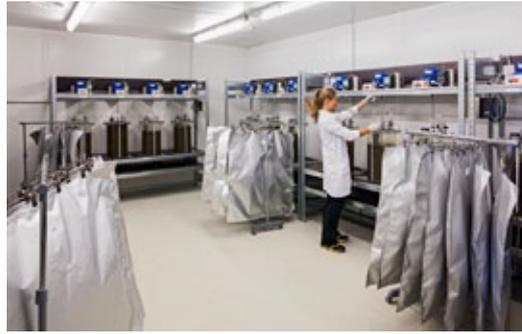
Continuous biogas model plant with 36 fermenters
