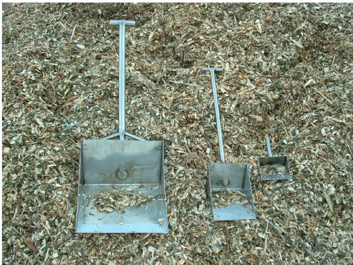
Figure 1. Recommended sampling equipment for taking solid biofuel samples (From Burvall et al, 2010).
