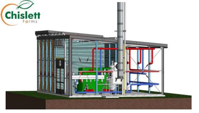
BIOHOUSE – All aspects are first designed and CAD modelled in 3D including the building, the mechanical plant, hydraulics, fuel storage and handling
