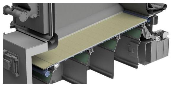
Windsor manufactured water-cooled vibrating grate coupled with windswept spout feeders, offers an optimal solution for biomass combustion. This grate provides a combustion plant that is flexible, automated, and able to ensure that steam pressure remains within specified limits during all stoking and grate actions.
